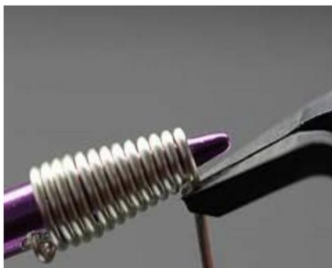
Poke the 16 gauge wire through the hole opposite where the 20 gauge wire went in; shove the wire through the hole, pushing the 20 gauge wire out.
