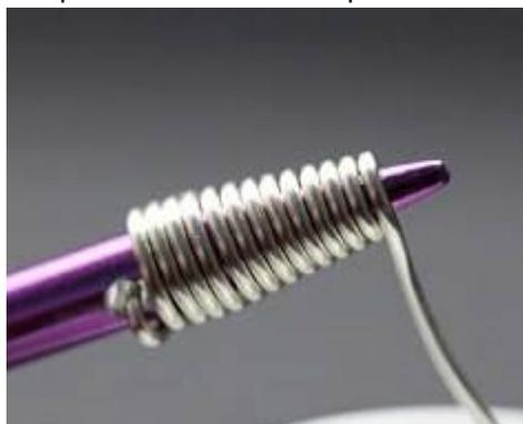
Using flush cutters, cut wire close to last curve of coil.
