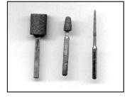
After annealing and soaking in soapy water, your thimble will practically pop right off the mandrel – much easier than removing a bead! These are the Dremel tools I use to clean the side walls, clean the inside of the top and drill the hole.
